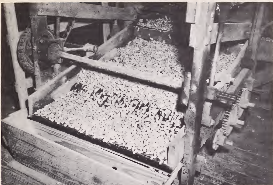
FIGURE 13.—A stemming machine—Peanuts are passed through revolving serrated disks which cut off any stems not removed in the picking operation.
